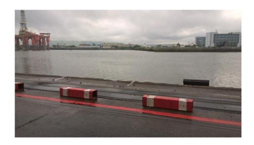
All Quay users are advised that it is Harbour Policy that lifejackets of minimum buoyancy of 150N MUST be worn by all personnel working to the water side of the red lines marked on the quay. Where no line is marked, life-jackets MUST be worn within 2m of the quay edge.
